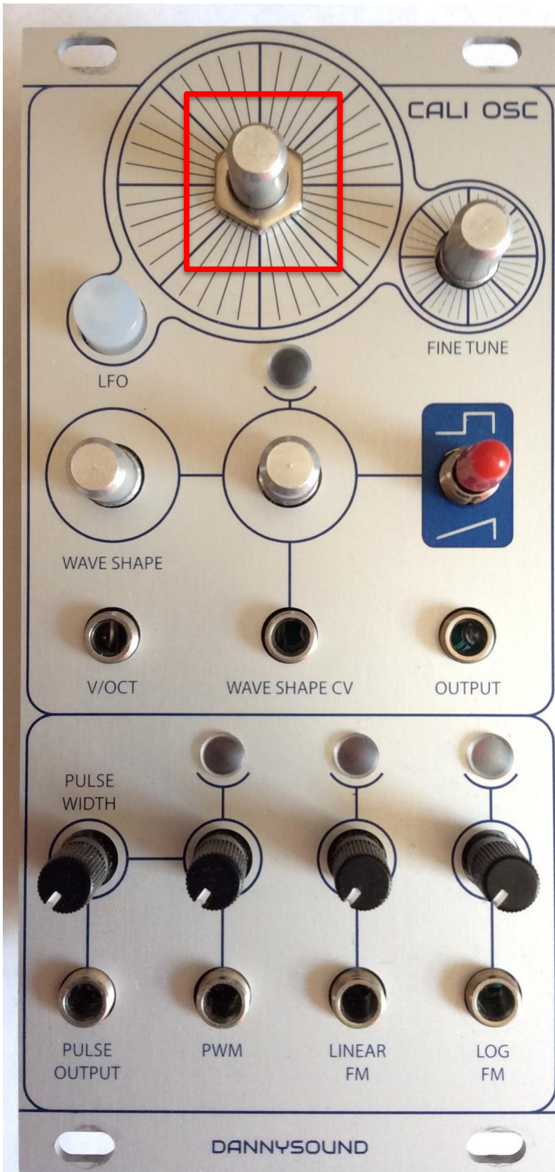
30 – Fit the panel and insert second pot nut but do not fully tighten.
