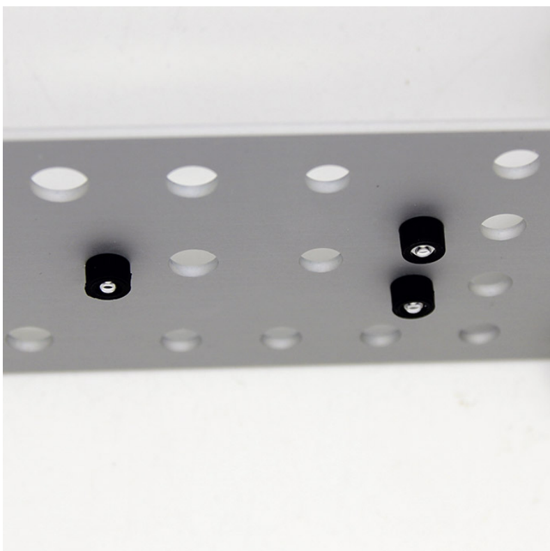
28 – Insert LED light pipes and retainer clips
