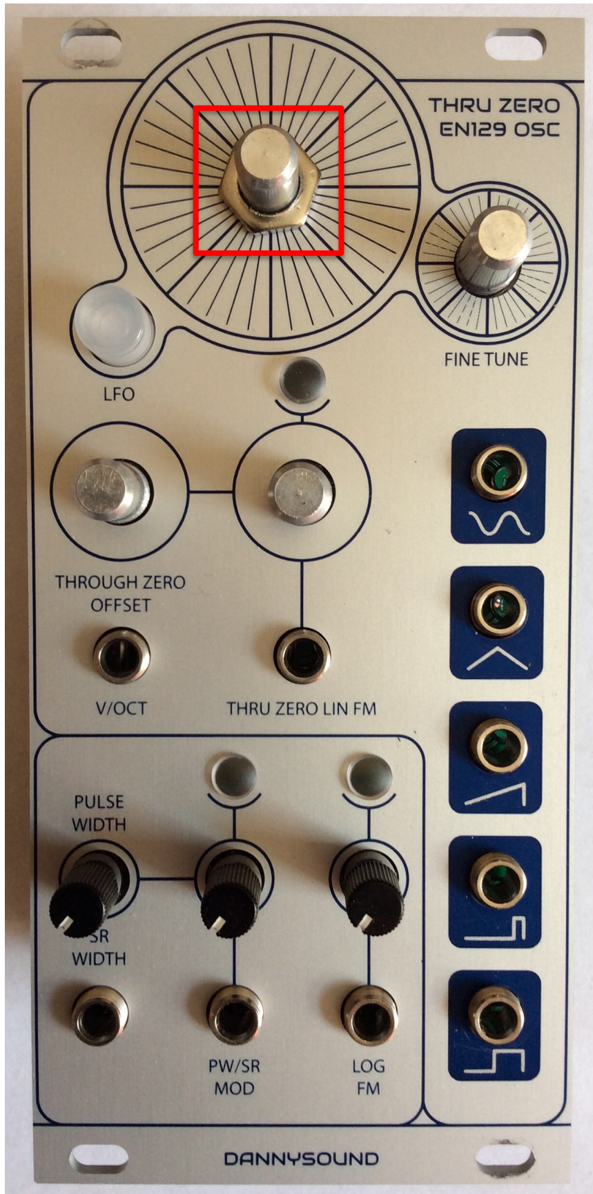
29 – Fit the panel and insert second pot nut but do not fully tighten.
