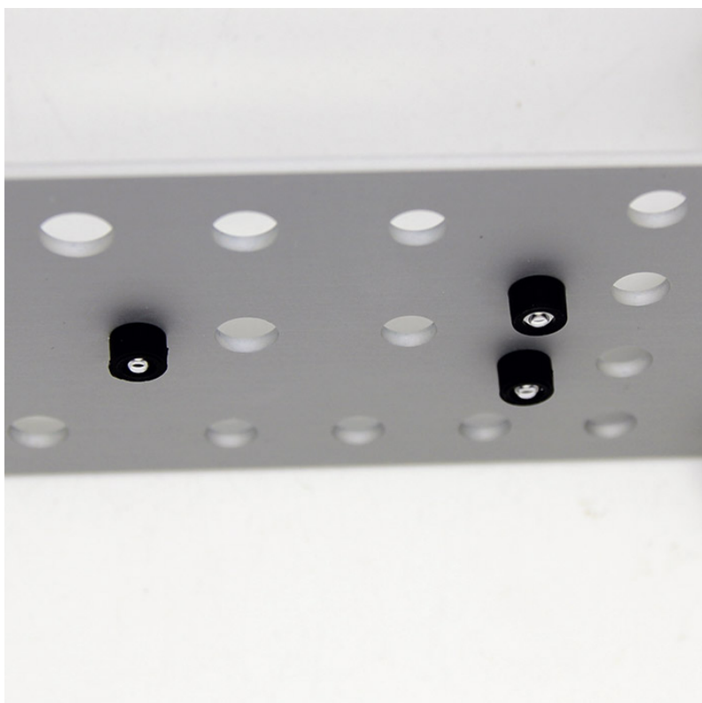
28 – Insert LED light pipes and retainer clips
