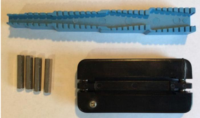
The blue bending gauge is for bending the resistor and diode legs to the right size. The black IC straightener is for straightening pins of op-amps etc. The silver standoffs are 25mm Female to Female.
