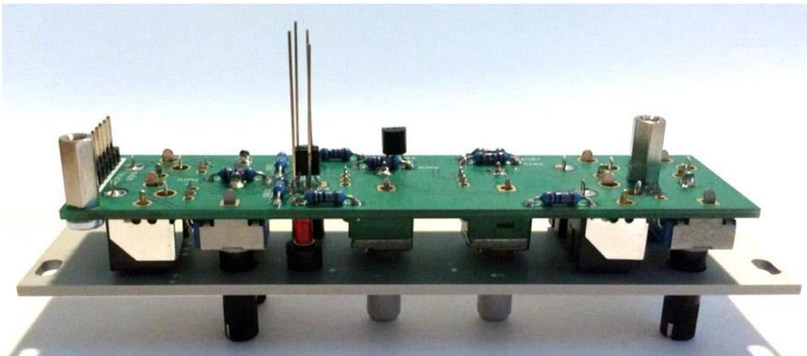
48 – Solder one leg of each of the LEDs, you can then reflow the solder to that pin while holding the LED legs to position it against the light pipe.
