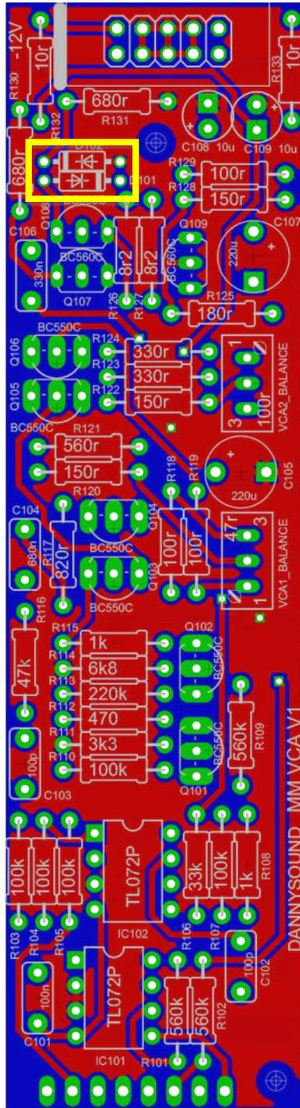
19 - 2 x 1N4148 (D101, D102) **NOTE:** orientation of this part is vital - be sure to match the line on the component with that on the PCB silkscreen
