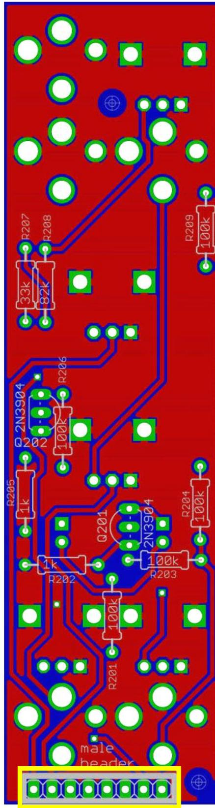
41 - MALE 1x8 pin header – this header is placed on the **same side** of the PCB as the resistors and transistors
