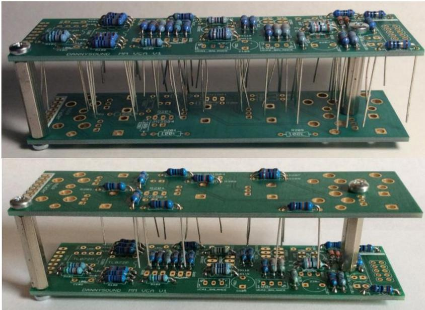
The top picture is for stuffing the Outer Board. It has the advantage of being much quicker to place all the resistors etc and it's easy to fix any mistakes. You can then solder everything from the top in one go (make sure you have decent temp. solder iron with not too fat tip!). Then unscrew the standoffs and clip all the legs. Reverse both boards as in the lower picture for the Pots Board.
