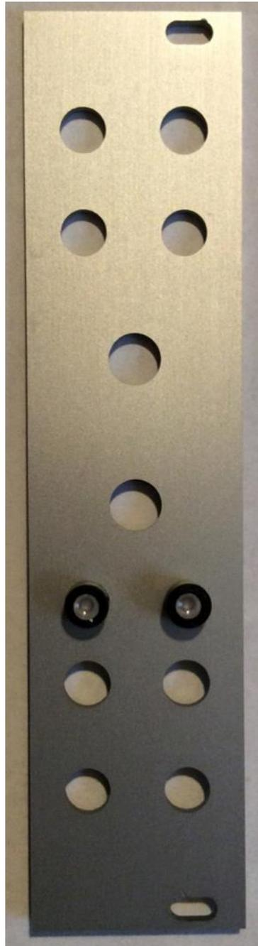
43 – Install 2 x Light pipes and retaining clips
