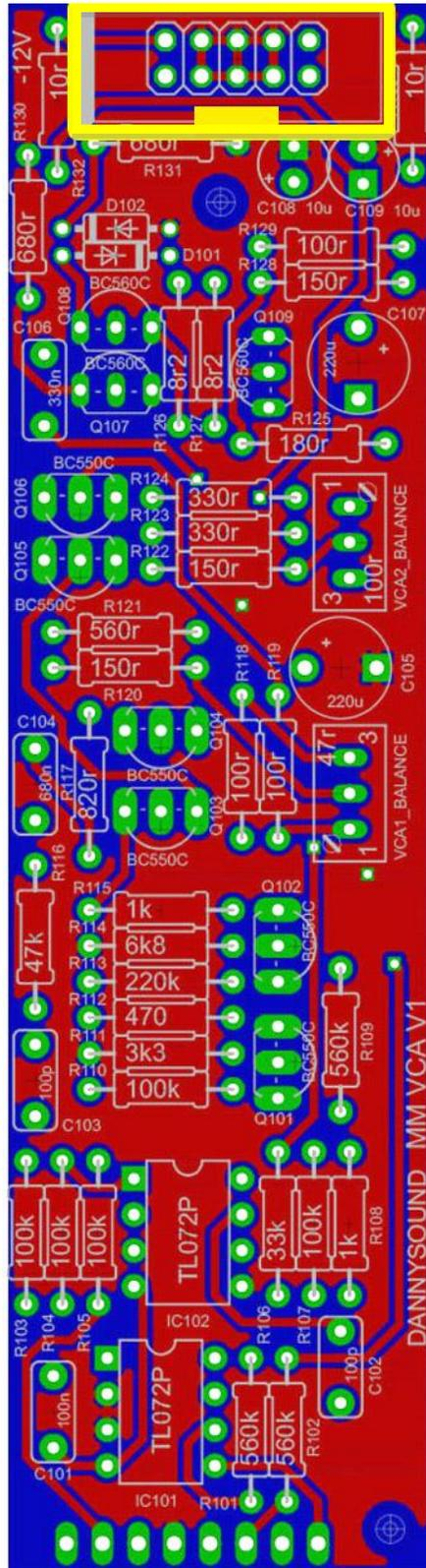
33 – 1 x SHROUDED 2x5 pin header - **make sure the slot is facing away** from the edge of the PCB as indicated above. Orientation is vital!
