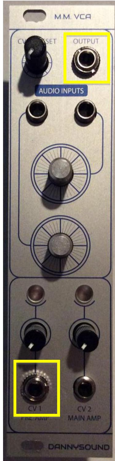
47 – Fit the panel in place, then while holding everything together turn over and solder one pin of the lower CV 1 jack socket and one pin of the output jack socket.
