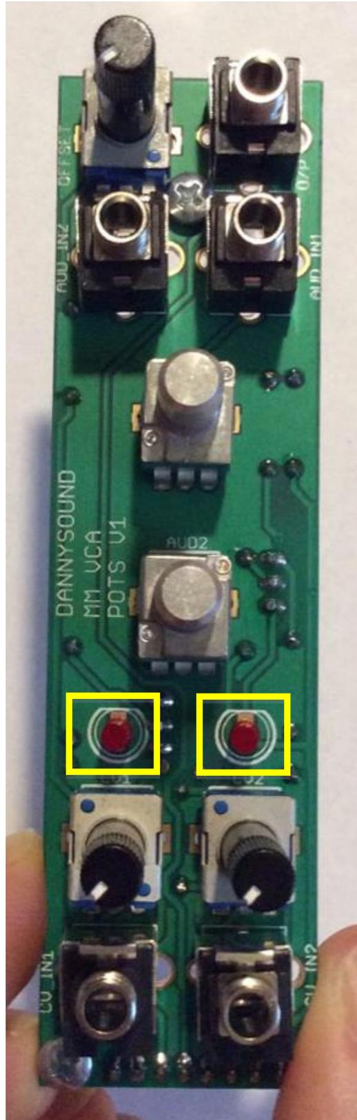
46 - 2 x 3mm Red LEDs - **NOTE:** orientation is vital, the shorter leg of the LED should go to the square pad and flat side of the PCB silkscreen diagram.
