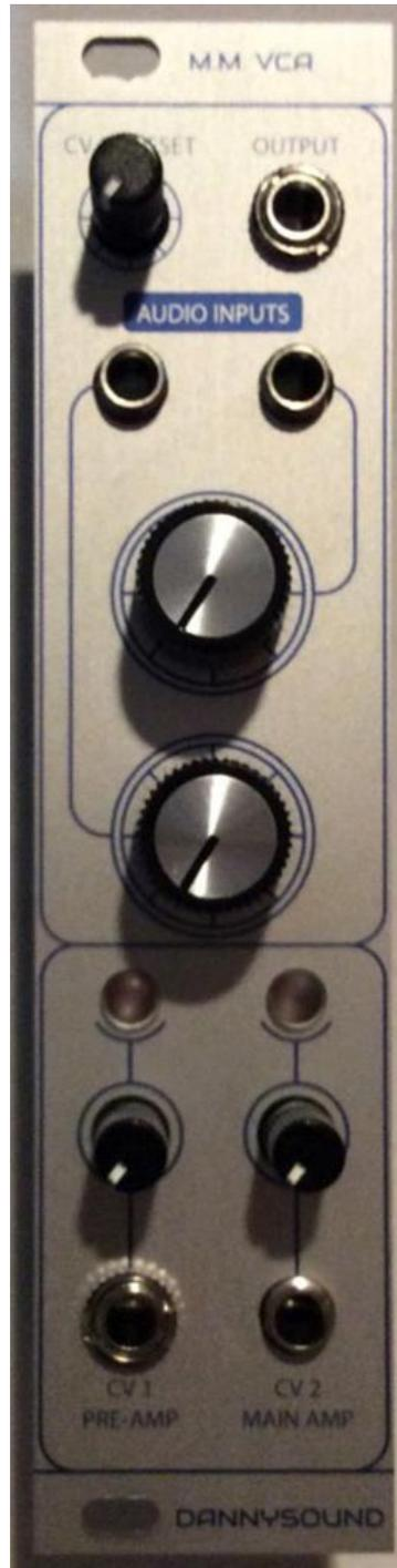
49 – Add the knobs then solder one of the ground tabs of each pot (including the tall trimmers). There is a little room for adjustment of the tall trimmers and pots so if they look out of alignment against the graphics or if the tall trimmers slightly rub when turn them you can reflow the solder whilst applying a little pressure to get them positioned perfectly.
