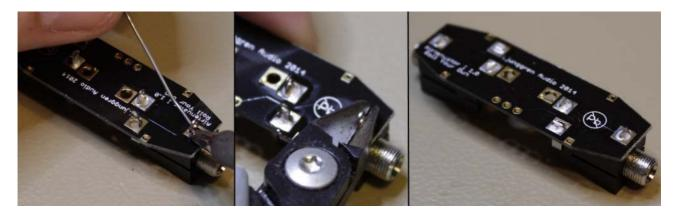
Solder the potentiometer. It can help to bend the wide leads a little to fixate the potentiometer in place before soldering. A PCB holder with crocodile clips holding around one jacks bushing is helpful. Cut off the leads after soldering.
