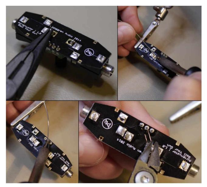
Optional step if you use no-clean flux. Clean off the flux carefully without getting flux cleaner in the potentiometer. Apply the flux cleaner to a cotton tip or similar and then use the cotton tip for rubbing the flux. Wipe clean after with some dry low lint paper or cloth. A video showing the final cleaning step can be found here: <u>http://youtu.be/dysoSpufuGU</u>
