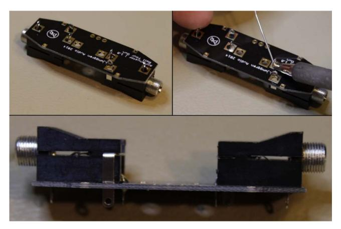
Solder the rest of the leads after you checked that the jacks are flat against the PCB. Cut off the leads after soldering.
