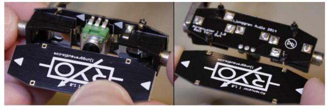
Solder the pins to the Cover PCB.
