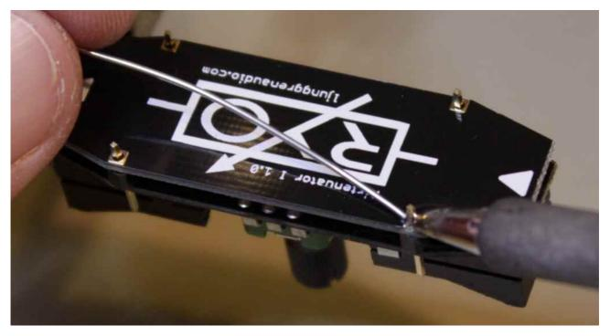
Before you solder the pins on the Main PCB. Make sure one last time that the triangle-arrows are pointing the same way on both sides.
