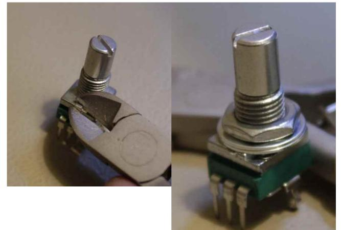
Place potentiometers, jacks, switches and LED in their positions but wait with soldering until the front panel is mounted.
