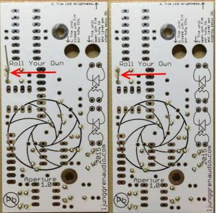
Solder regular sized (ca 7mm) resistors. Resistors are not sensitive to mounting direction.
