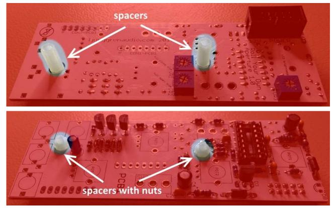
Put the pin & socket strips into each other. Place them between PCB1 and PCB2 in their respective places. **Take a firm grip with a plier around the spacers and screw the screws into place like in the picture below.** It's important that the grip is firm as there is a bit of friction in this step and we don't want the nuts to loosen. If the nuts gets loose, tighten them again.
