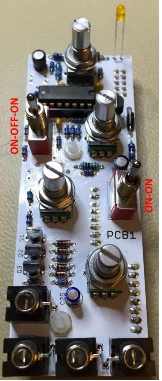
Place the front panel on top and add 1 washer and 1 nut to each potentiometer, jack and the switch. Use a socket wrench to avoid scratching of the frontplate.
