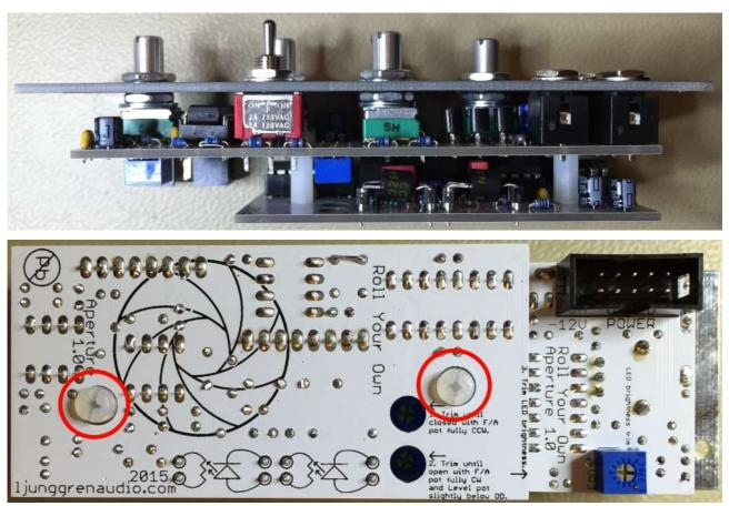
Mount the knobs. The big red knob will touch the front panel so you need to make sure there is a tiny gap under it. You can accomplish this with a bit of **thick paper or envelope** and cut out an opening for the potentiometer shaft. Remember to have a slot in the side of the paper so it can be removed after the knob is attached.
