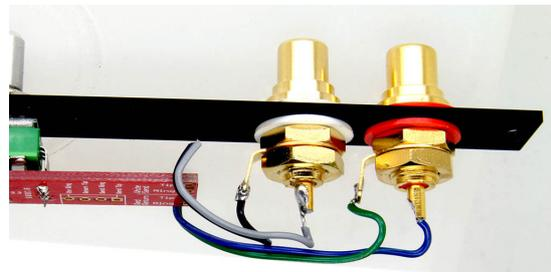
Here we show the **SEND RCA** soldered, the **black wire** on the ground ring is going to the PCB input marked **Ring**, the **grey wire** on the tip of the jack is going to the PCB input marked **Tip**.
