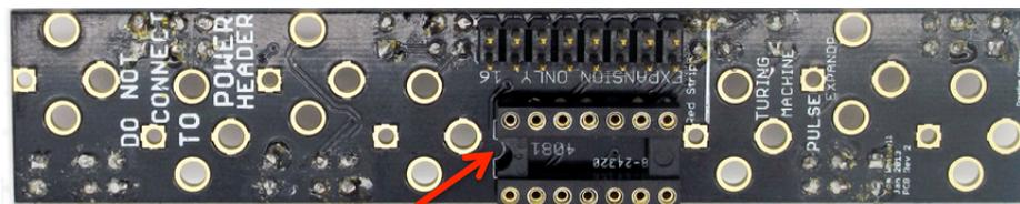
**TAKE CARE:** Ensure the notch in one end of the IC Socket is aligned with the silkscreen outline on the PCB.
